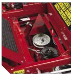
Quick removal of the floor pan provides convenient access to the top of the deck for easy cleaning and service.
