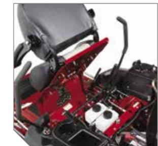
Flip-up seat provides easy access to serviceable components. Belt and blade part numbers are referenced under seat.
