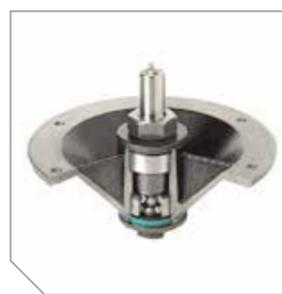
Hercules™ II Spindles industrial 10" dia. cast-iron spindle assembly with 1 3/16" dia. shaft and greaseable double row angular contact ball bearings, which can be greased through the convenient top access grease fitting.
