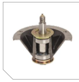
Cast-Iron Spindles longer usable life, 1" shaft with top access grease fitting for greaseable dual ball bearings, six-bolt 8" flange design adds strength and greater dispersal of energy to deck assembly. (61" models)
